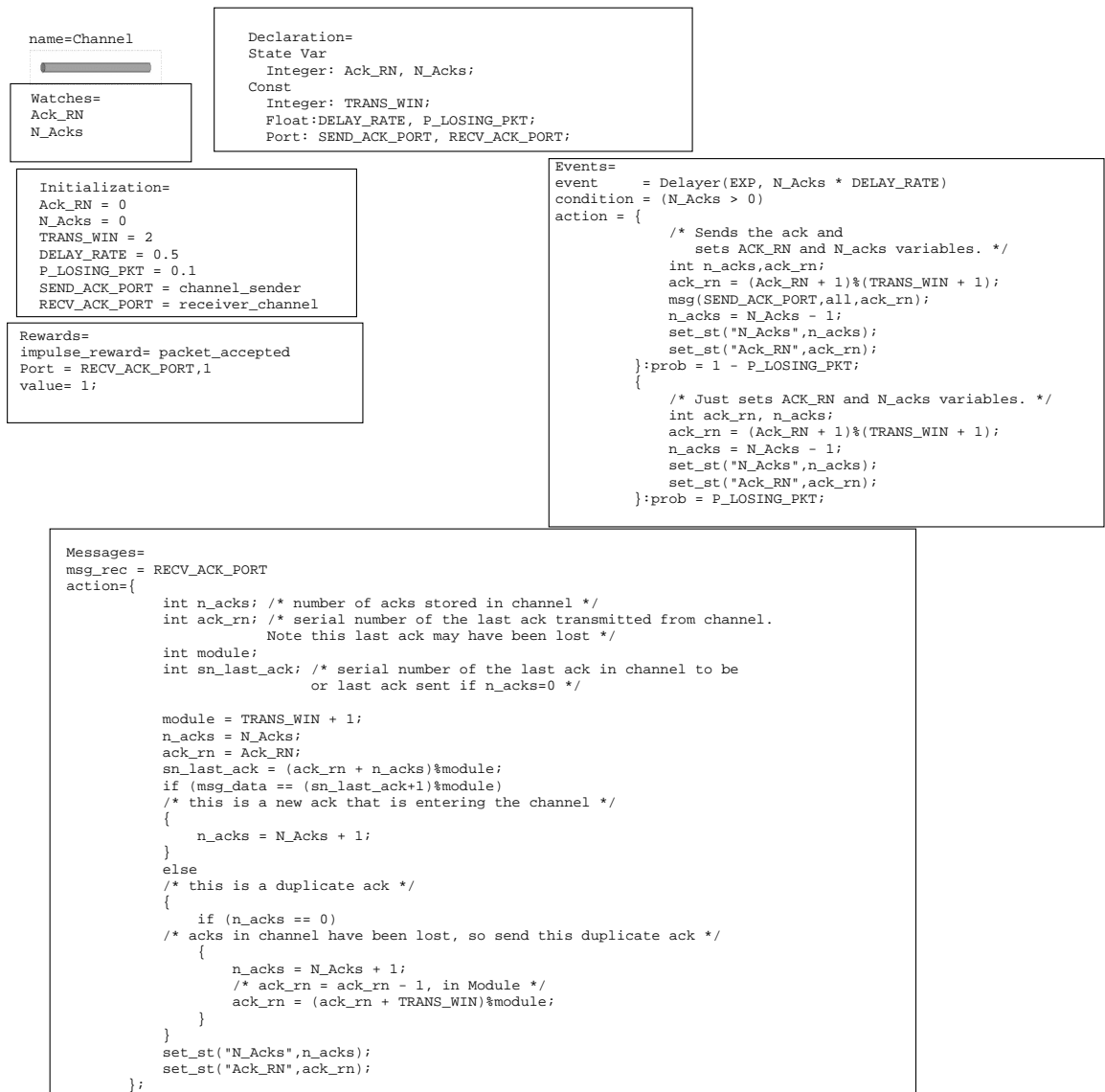
Figure 9.36: The Channel object (Go Back N Model). Model 1
