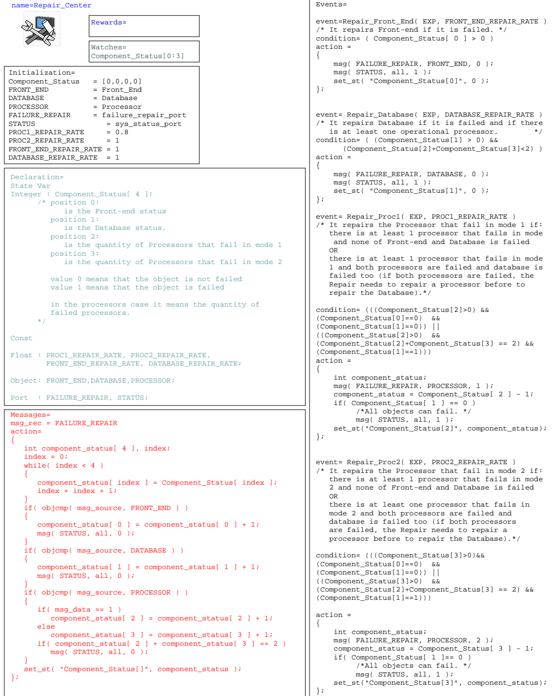
Figure 9.32: The Repair object (Database Model).
