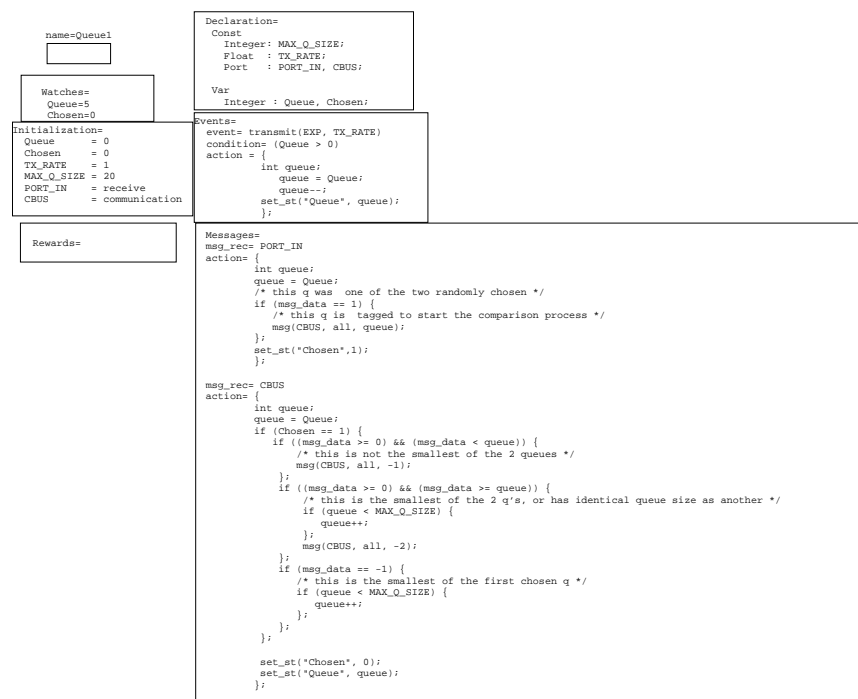
Figure 9.18: The Queue object (Multiple Action Model).
