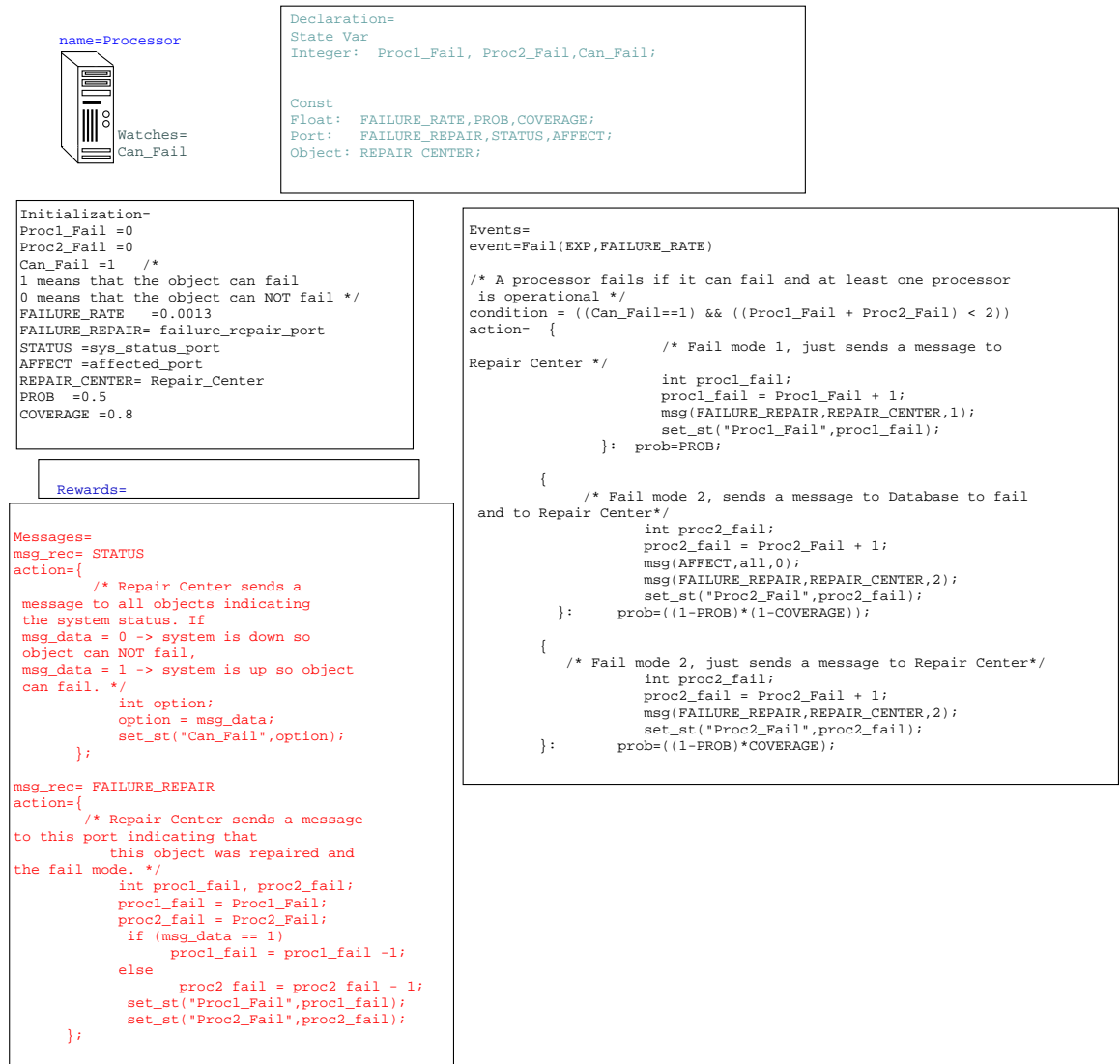
Figure 9.31: The Processor object (Database Model).
